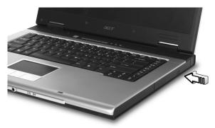
When the power is off, you can eject the drive tray by using the emergency eject hole.
