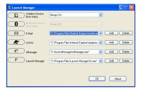
Launch Manager allows you to set the four easy-launch buttons located above the keyboard. "Easy-launch buttons" on page 9 for the location of the easy-launch buttons.
