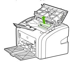
3. When you have removed the jammed media, replace the print cartridge, and close the print cartridge door.
