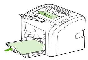
4. After side one has printed, gather the printed pages, turn the printed side down, and straighten the stack.
