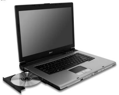
Insert a clip to the emergency eject hole to eject the optical drive tray when the computer is off.
