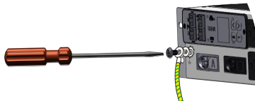
Figure 18. Grounding Screw Location for Horizontal Models
