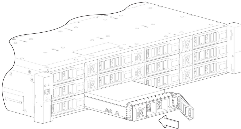
Figure 44. Installing an LFF drive carrier module (1 of 2)
