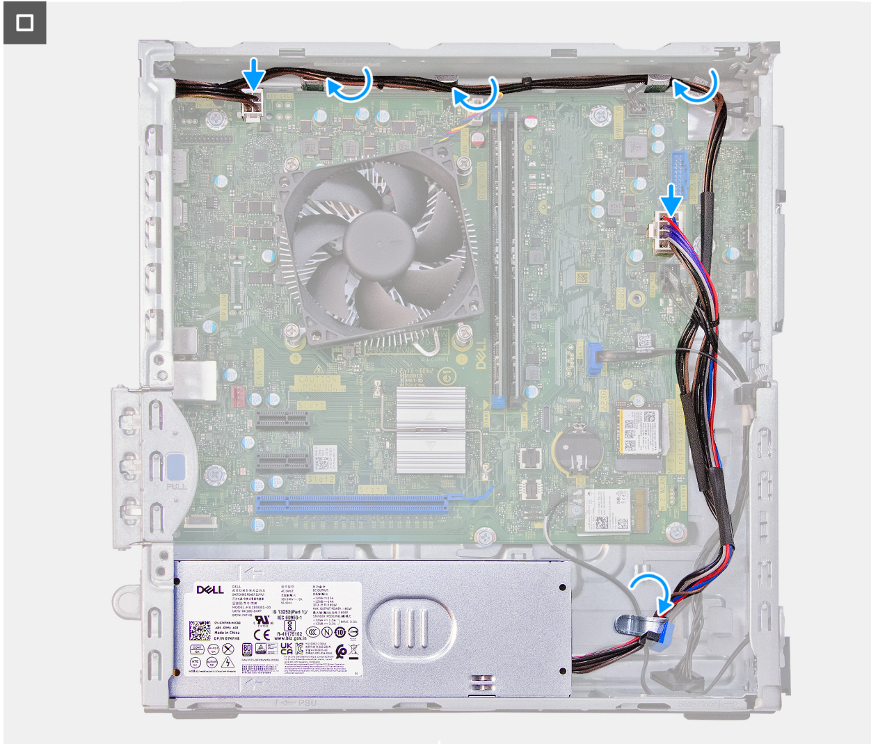
Figure 36. Installing the power-supply unit
