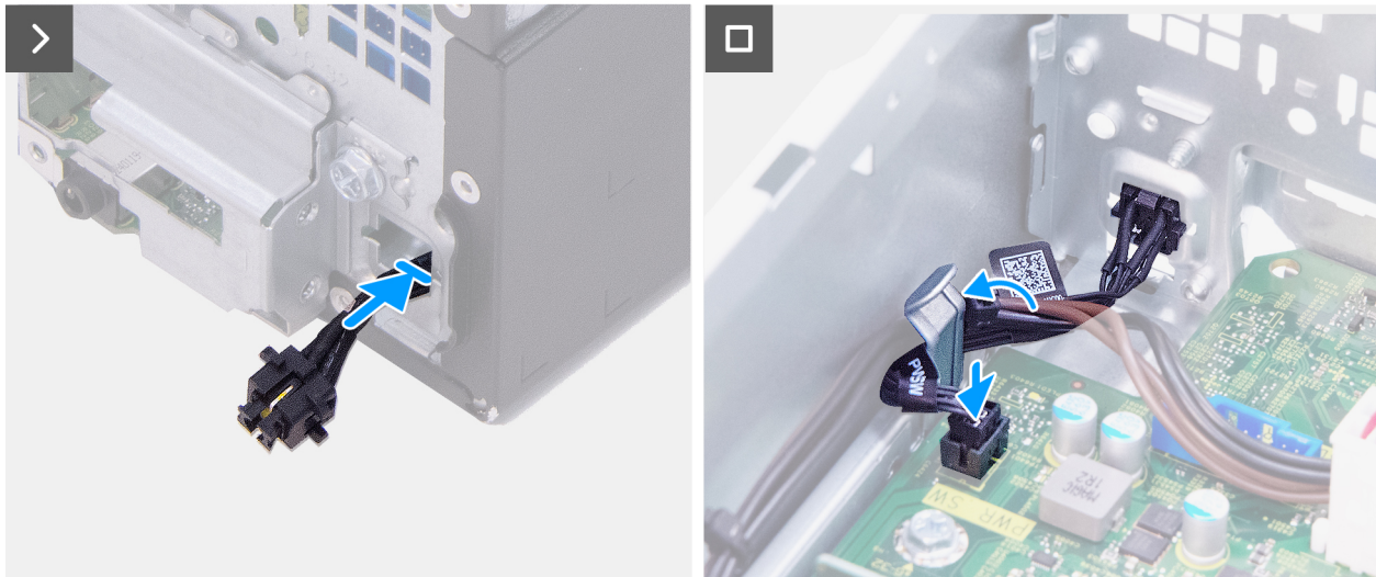
Figure 44. Installing the power button
