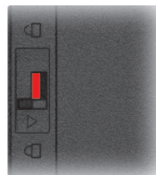
Incorrect (revealing red part)
