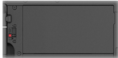
Incorrect (revealing red part)
