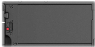
Incorrect (revealing red part)
