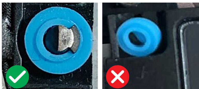
Figure 40. Seating position of the rubber grommets
