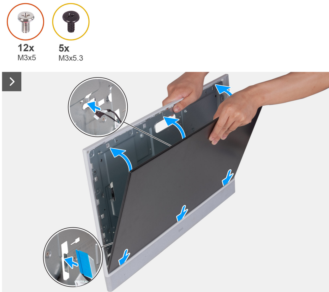
Figure 62. Installing the display panel
