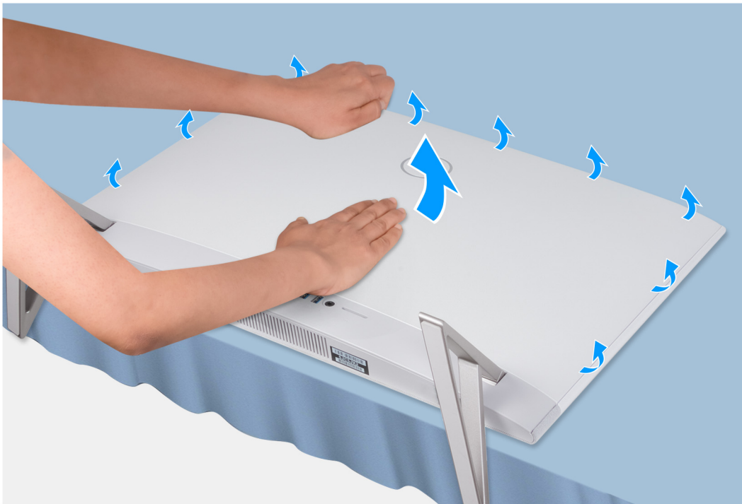
Figure 20. Removing back cover
