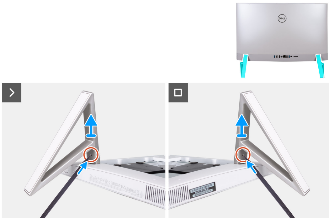
Figure 17. Removing the stand
