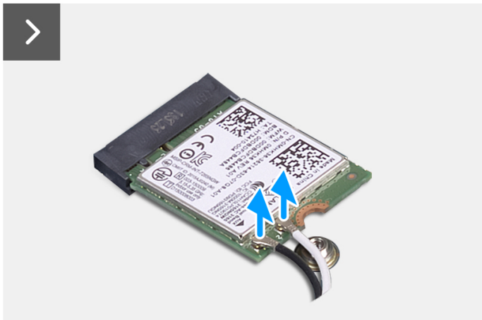
Figure 32. Removing the wireless card
