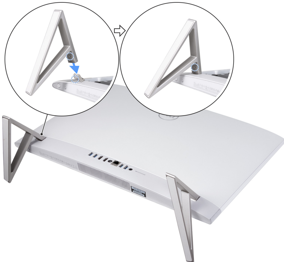
Figure 9. Install the stand
