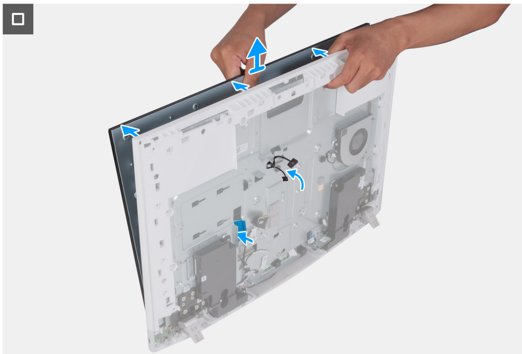
Figure 61. Removing the display panel
