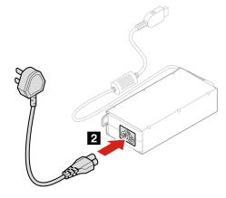
3. Align the two hooks on the power adapter bracket side with the two holes on the VESA mount bracket side. Push forward the power adapter bracket to secure it on the VESA mount bracket.
