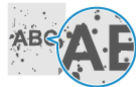
Toner smudges and splatters appear
