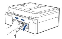
(MFC-J4555DW) Open the Jam Clear Cover (1) on the back of the machine.
