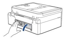
8. Put the paper support firmly back in the machine. Make sure you fit the paper support into the channels.
