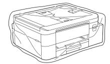
10. Pack the machine in the original carton with the original packing material as shown below.
