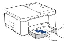
3. Lift the paper support (1), and then pull it at an angle completely out of the machine as shown by the arrow.
