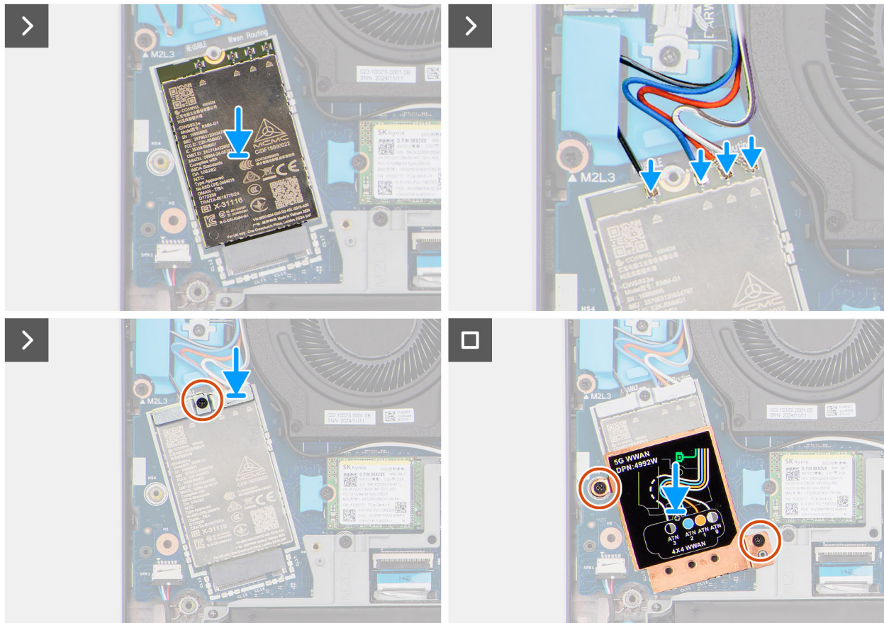
Figure 32. Installing the WWAN module
