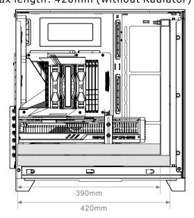
PSU length max length: 200mm (with 2.5" SSD) PSU length max length: 260mm (without 2.5" SSD)
