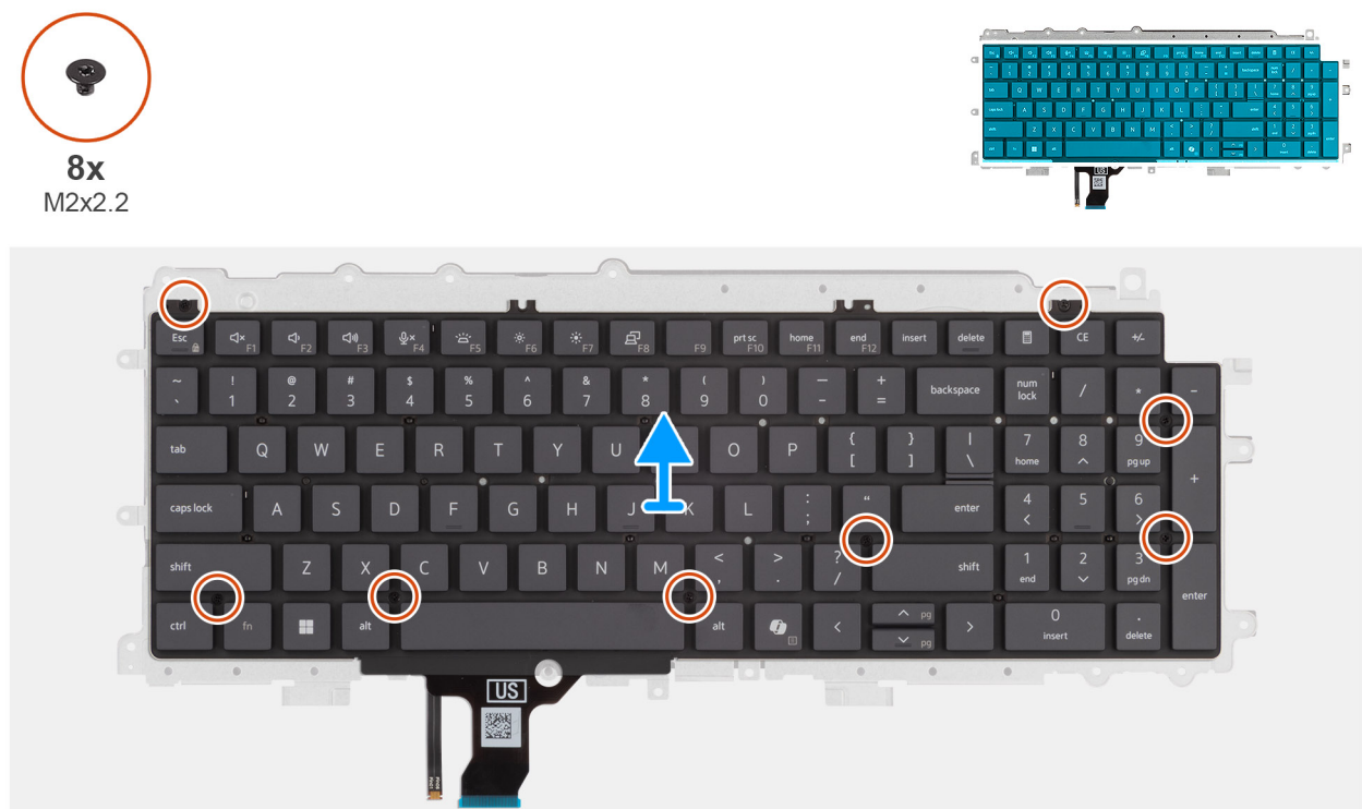
Figure 56. Removing the keyboard support plate
