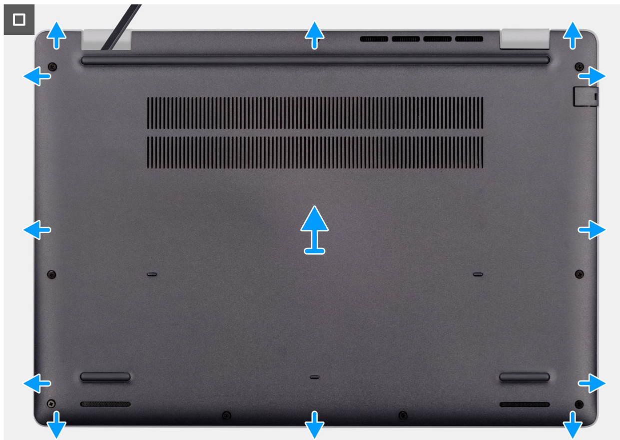
Figure 12. Removing the base cover
