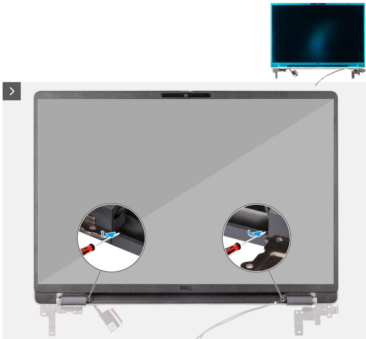
Figure 67. Removing the display bezel
