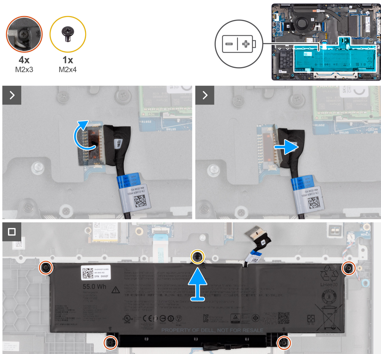
Figure 17. Removing the battery
