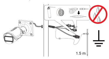
**8.** Assemble the waterproof shell around the Ethernet cable. Connect the Ethernet cable to the camera's RJ-45 connector.
