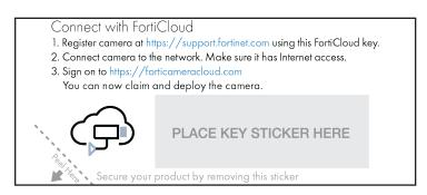
Remove the label from the camera. Keep it together with the serial number and MAC address for later identification. 4. Once the camera connects to the cloud and is claimed, its firmware will be updated automatically. This may take several minutes and multiple reboots. Do not power off the camera during this process.
