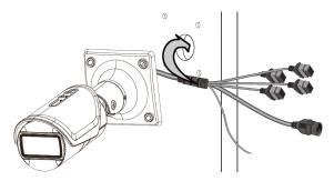
Allow slack in the cable so that any condensation will drip away from the waterproof seal, not towards it.
