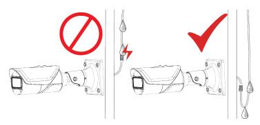
**6.** Plug in any required pigtail cables except for the power supply. (Do not connect the power supply until the ground wire is connected, as shown in the next step.)
