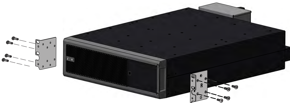
Figure 21. Rack Ear Installation
