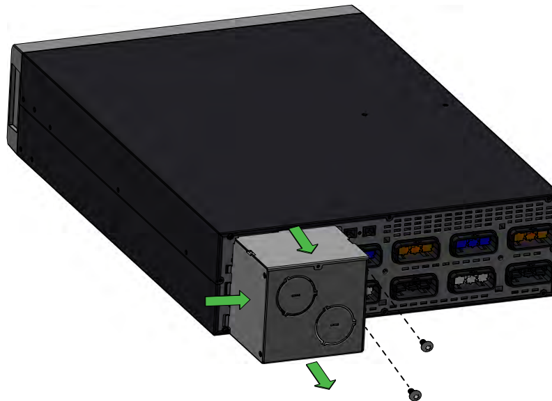
Figure 23. MBP20KIUPARA AC Terminal Wiring Box Removal
