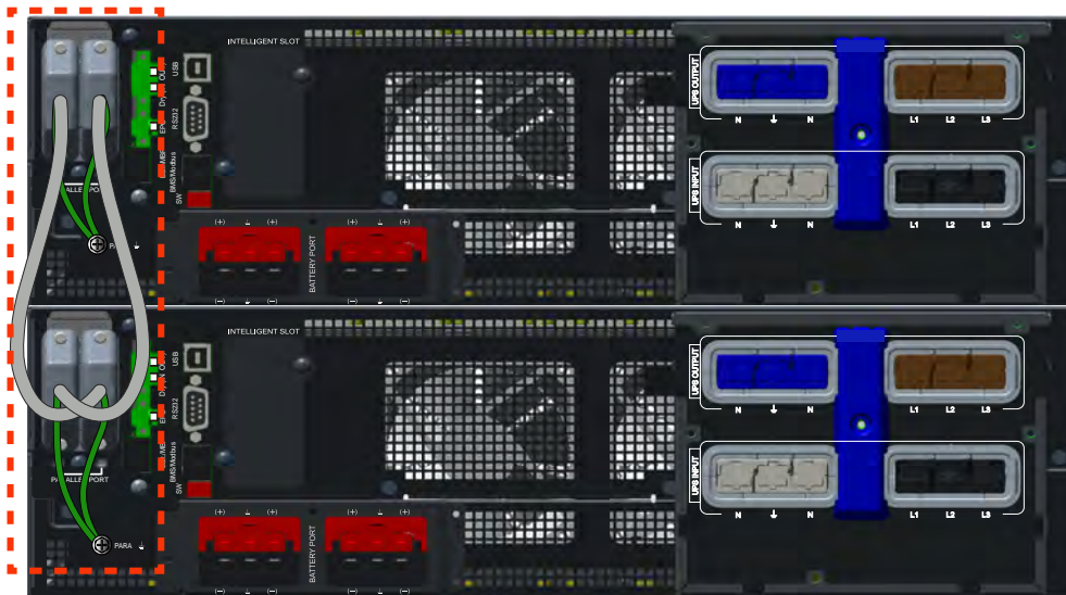
Figure 36. Connecting the Parallel Cable
