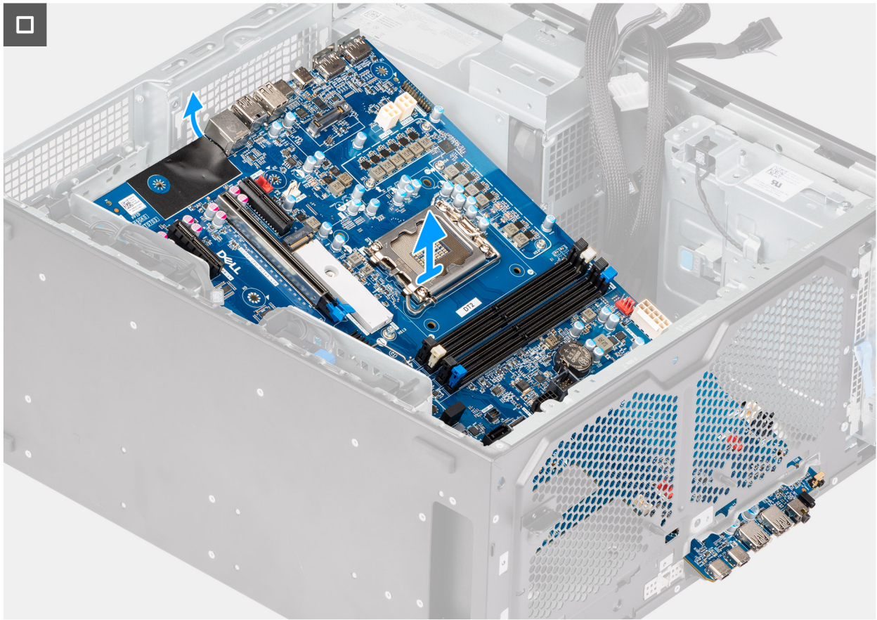
Figure 92. Removing the system board
