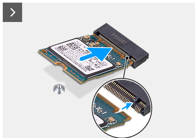
Figure 32. Installing the M.2 2230 PCIe solid state drive
