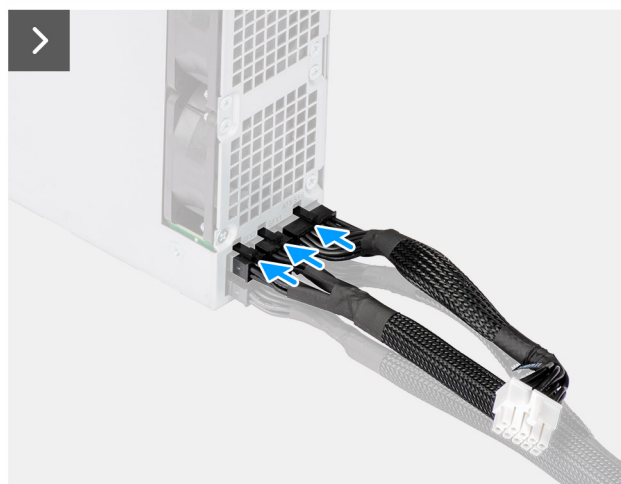
Figure 55. Installing the 1500 W power-supply unit
