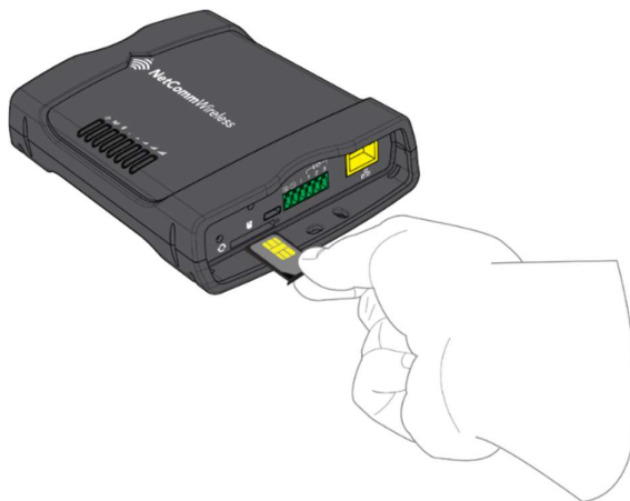
Figure 17 – Inserting the SIM card
