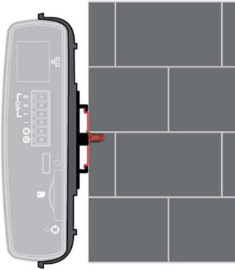
Figure 9 – Wall mount with DIN rail mount adapter
