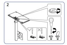
Tightly fasten the connecting screw at the bottom of the stand base. Fasten the large screw in the middle for assembly.
