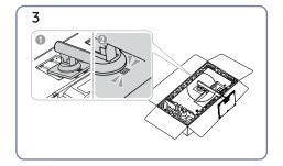
Push the assembled stand into the main body in the direction of the arrow as shown in the figure.
