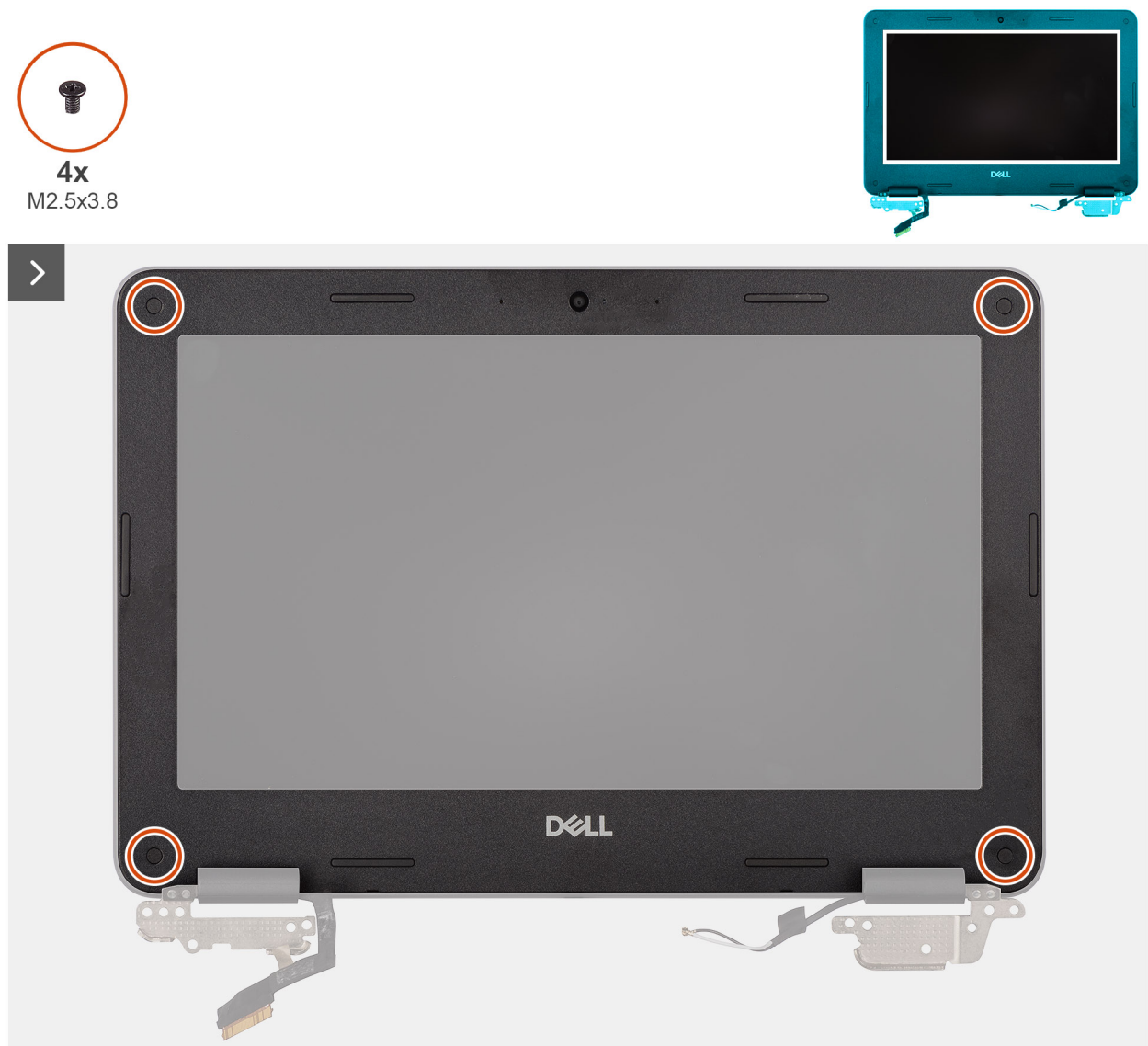
Figure 49. Removing the display bezel
