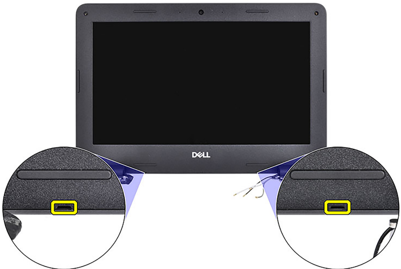
Figure 52. Pry the display bezel from the two recesses near the hinge caps
