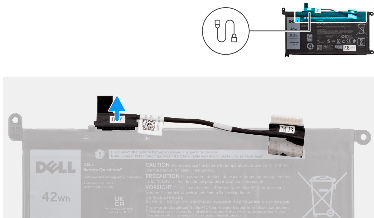
Figure 22. Removing the battery cable
