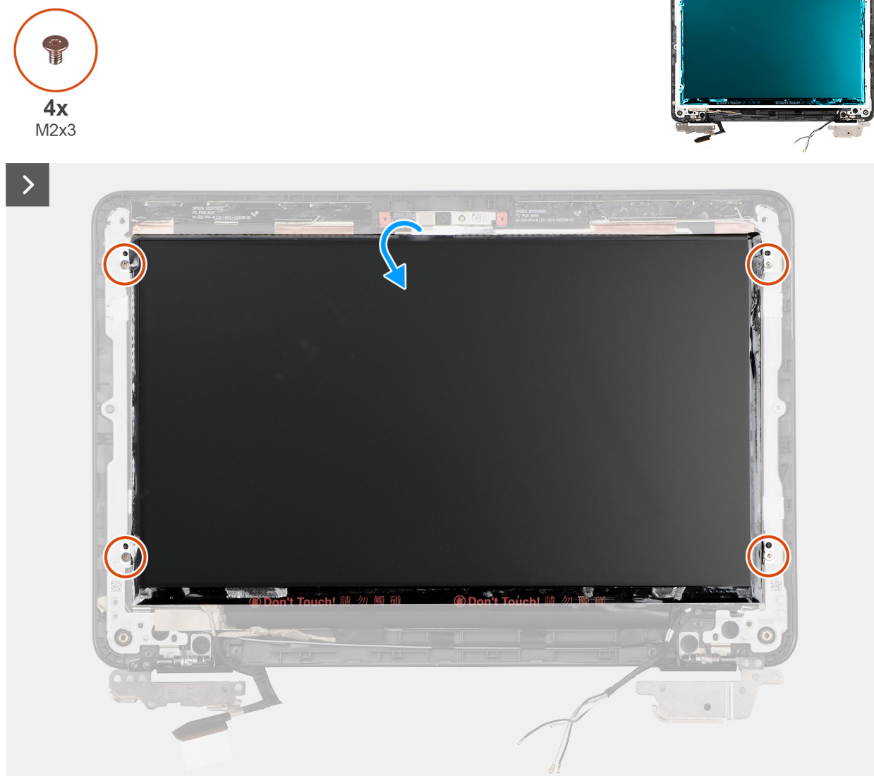
Figure 59. Removing the display panel
