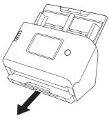
The document eject tray can be adjusted to 3 lengths. Pull out the document eject tray according to the length of the document. Also, erect the document eject stopper on the front edge if necessary.
