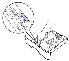
5. Wipe the two pick-up rollers inside the machine to remove dust.
