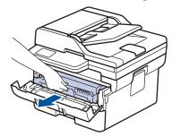
3. Clean the corona wire inside the drum unit by gently sliding the green tab from left to right and right to left several times.
