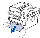
Pulling the jammed paper downward using both hands allows you to remove the paper more easily.
