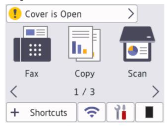
The warning icon • appears when there is an error or maintenance message; press the message area to view it, and then press to return to Ready Mode.
