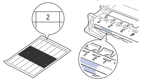
13. Turn the drum unit edge toward you while looking at the drum surface to find the mark.
