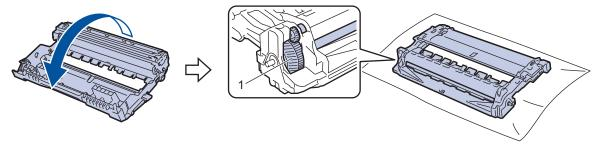
10. Use the numbered markers next to the drum roller to find the mark on the drum. For example, a dot in column 2 on the check sheet means that there is a mark in drum region "2".
