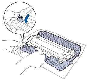
11. Turn the drum unit as shown in the illustration. Make sure that the drum unit gear (1) is on the left side.
