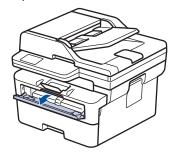
3. Use both hands to slide the manual feed slot paper guides to fit the width of the paper you are using.
