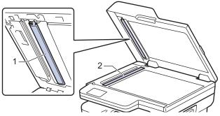
4. (For automatic 2-sided scanning models) Open the scanner glass cover (1), and then clean the other white bar (2) and scanner glass strip (3).
