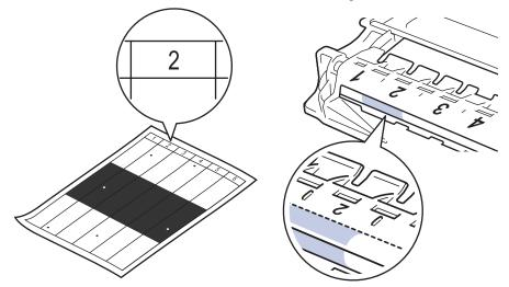
11. Turn the drum unit edge toward you while looking at the drum surface to find the mark.
