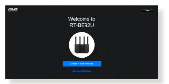
2. The wireless router automatically detects if your ISP connection type is **Dynamic IP**, **PPPoE**, **PPTP** and **L2TP**. Key in the necessary information for your ISP connection type.
