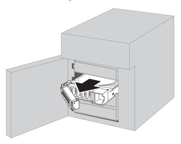
$\boldsymbol{5}$  Insert the new drive into the empty slot with the lock mechanism remaining open.
