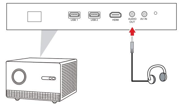
**NOTE:** If using headphones, it is recommended to use headphones with an impedance of 32 ohms or higher.
