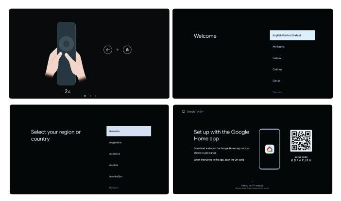
NOTE: To put the remote control in pairing mode, press and hold the Return (←) and Home (介) button until the remote control led indicator starts flashing.
