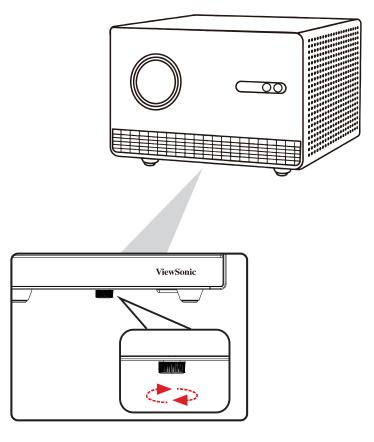
**NOTE:** If the projector is not placed on a flat surface or the screen and the projector are not perpendicular to each other, the projected image can become trapezoidal. However, the "Auto Keystone" function will correct the issue automatically.
