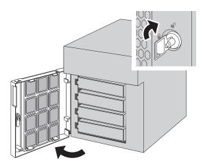
**2** Remove the front cover while holding the hook downward.
