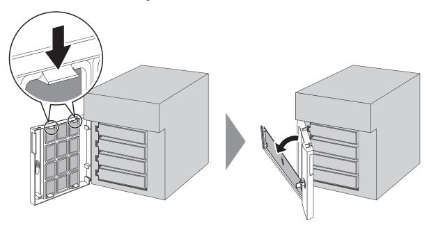
Remove the dustproof filter from the front cover and clear any dust, such as by using a vacuum cleaner.
