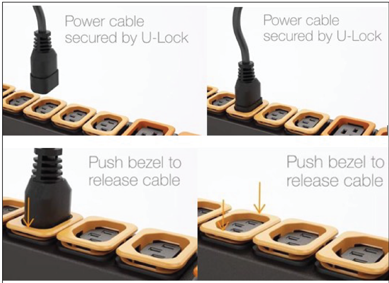
Figure 3.15 U-Lock Cord Retention Operation
