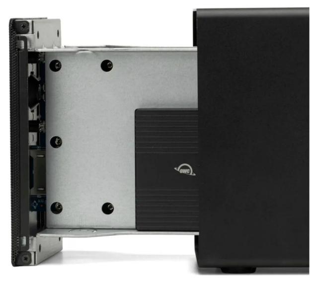
**5.** Secure the outer and inner chassis using the screws removed in Step 1.
