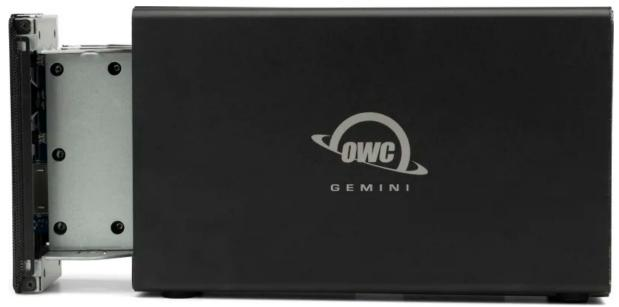
**2.** Set the inner chassis flat on the work surface and place a 3.5"/ 2.5" SATA or U.2 drive/adapter into the drive housing. The label should be facing upwards. Carefully seat the drive. Minimal force is needed.
