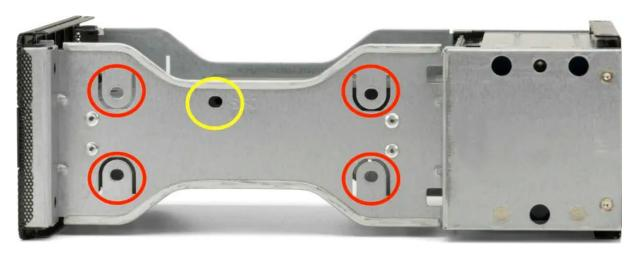
**4.** Ensure the ports on the back of the inner chassis and the port cut-outs on the back of the outer enclosure are oriented the same way, then slide the inner chassis into the outer enclosure so that the chassis' front plate is flush with the cover's front edge.
