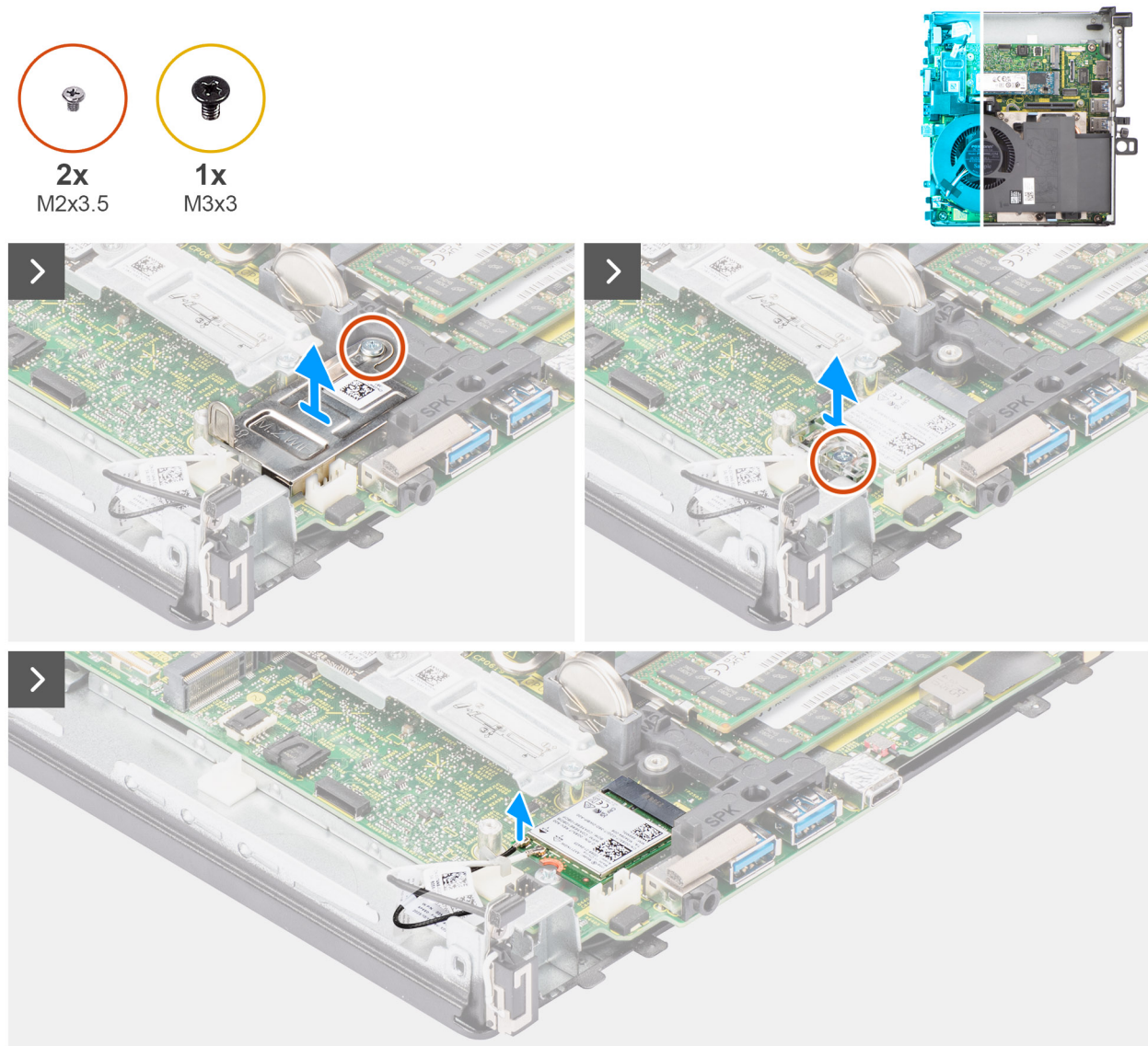
Figure 54. Removing the internal antenna—location 2
