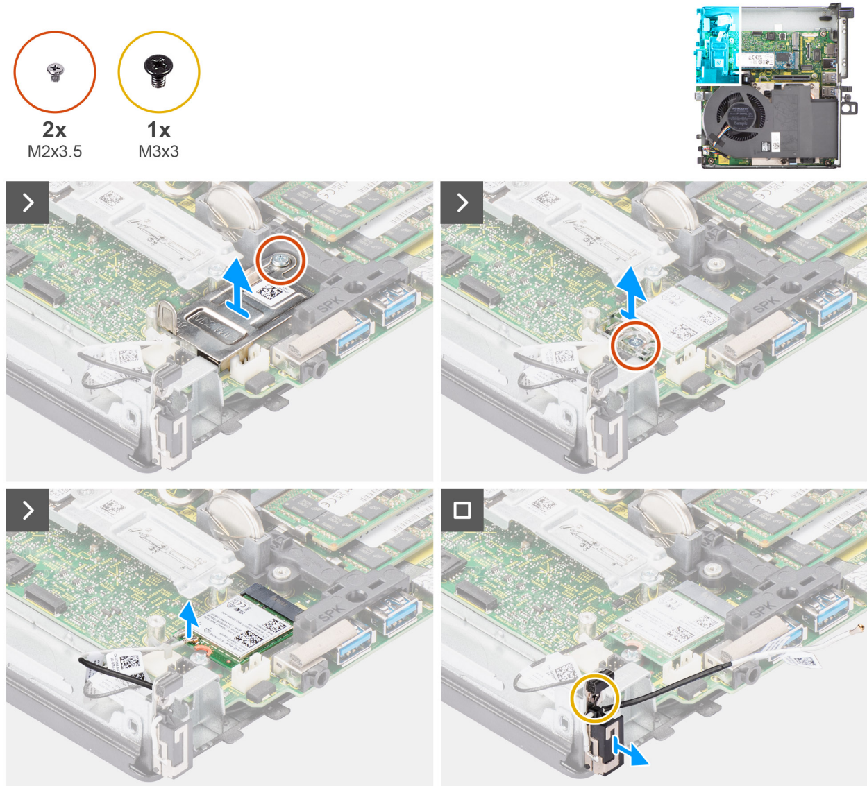
Figure 52. Removing the internal antenna—location 1
