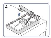
Stand upward to remove it in the direction of the arrow.
