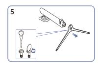
Remove the stand neck from the stand base by pulling it in the direcctiion of the arrow as shown in the figure.
