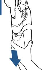
Turn the vacuum OFF and hold it vertically, pressing the Dirt Tank release latch. Gently pull the Dirt Tank from the hand vacuum.
