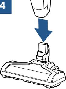
Secure the Removable Floor Nozzle back into the hand vacuum.
