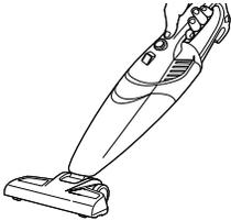
The Removable Floor Nozzle may be used with the hand vacuum for multi-purpose cleaning. To attach the nozzle, insert it into the opening at the bottom of the Dirt Tank. Press firmly to secure in place.
