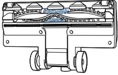
Turn the Removable Floor Nozzle over to remove any debris or to clear a clog in your Brush Roll.
