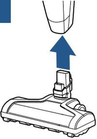
Make sure the vacuum is OFF. Press the release button to disconnect the Removable Floor Nozzle from the hand vacuum.
