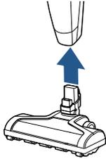
Then, attach the Removable Floor Nozzle by inserting it into the opening at the bottom of the Dirt Tank. Press firmly to secure in place.
