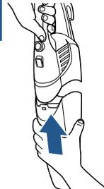
Replace Filter. Attach Dirt Tank to vacuum by securely fitting onto hand grip. Make sure Dirt Tank is correctly secured.
