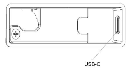
Note: The cable guard cover is secured by screws. You need to remove it before inserting the cable, and then install the cover and secure the screws after inserting the cable.
