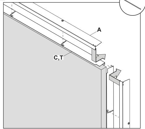
ENG Attach covers with nut bar inside cover. Displays not shown for clarity.
