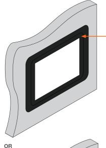
Press a finger into the top right corner. The left side of the panel will pop out and the panel can be removed.
