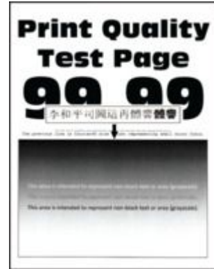
Fine lines are not printed correctly on page 518
