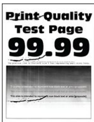
Repeating defects on page 534
