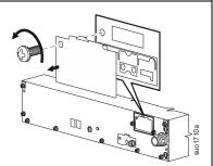
3 Connect the battery connector and communication cable.
