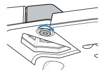
**1.** Route the USB cable from the CFS through the opening in the MP72, ensuring the cable is vertical in the pole slot.
