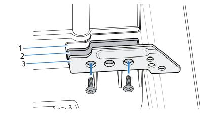
**3.** Insert the CFS filler cap and hold in place.
