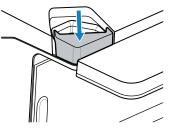
4. Install the filler cap screw and tighten until the filler cap is fully seated.
