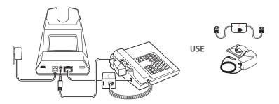
**IMPORTANT** Cisco phones use configuration  ${\bf D}$  on the bottom of the base. Most other phones use the default configuration  ${\bf A}$ .
