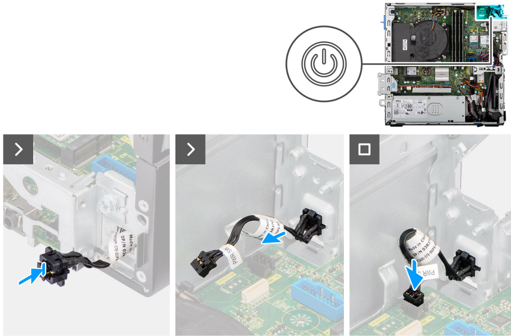
Figure 34. Installing the power button
