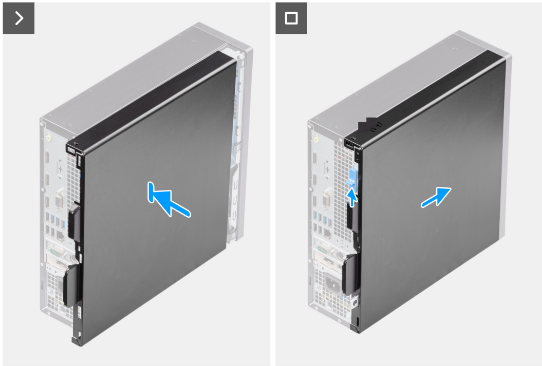
Figure 4. Installing the side cover
