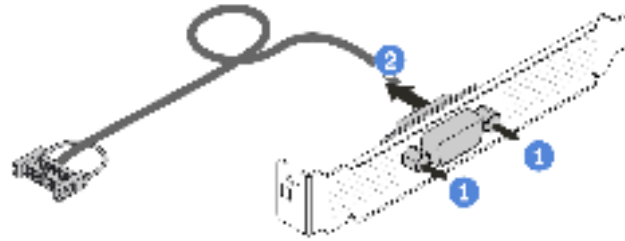
Figure 186. Disassembling the serial port module
