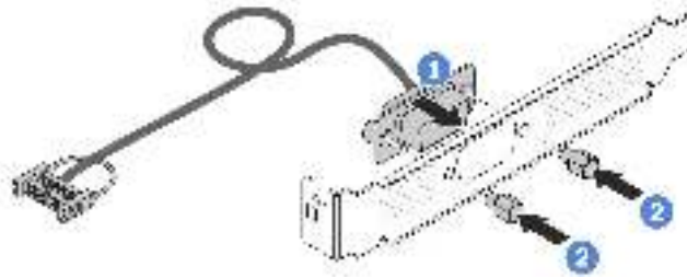
Figure 187. Assembling the serial port module
