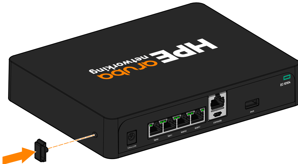
Figure 5 Attaching a Cable Saddle
