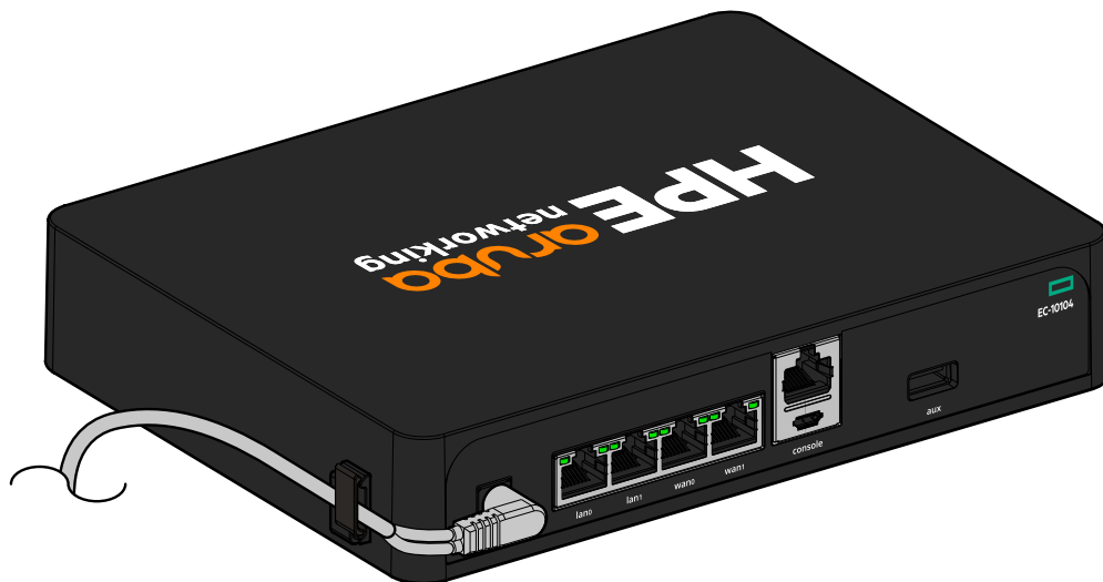
Figure 6 Securing a Cable
