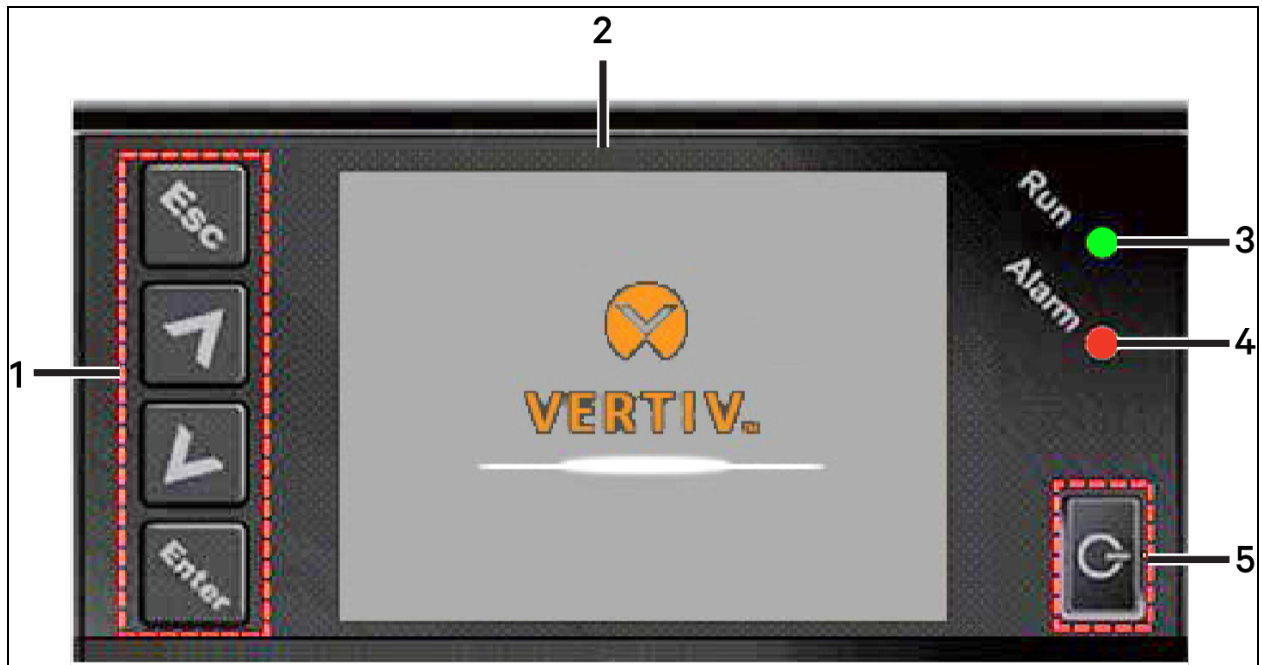
Figure 3.1 ITA2 Control Panel
