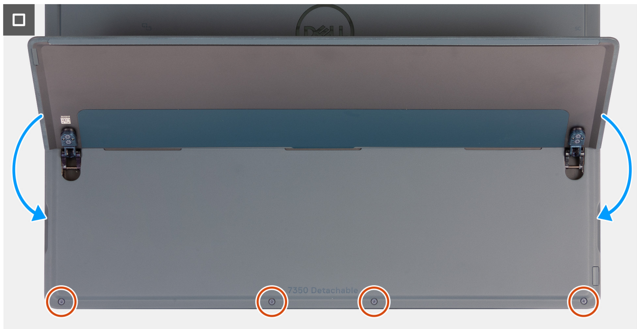
Figure 23. Installing the display assembly
