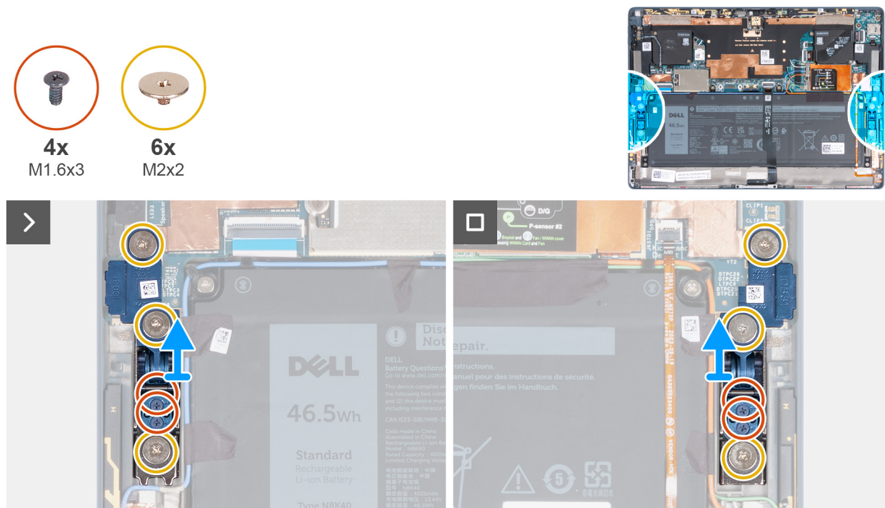
Figure 55. Removing the kick-stand hinges
