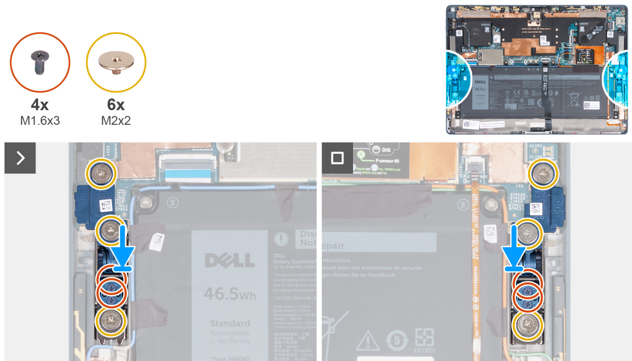
Figure 56. Installing the kick-stand hinges
