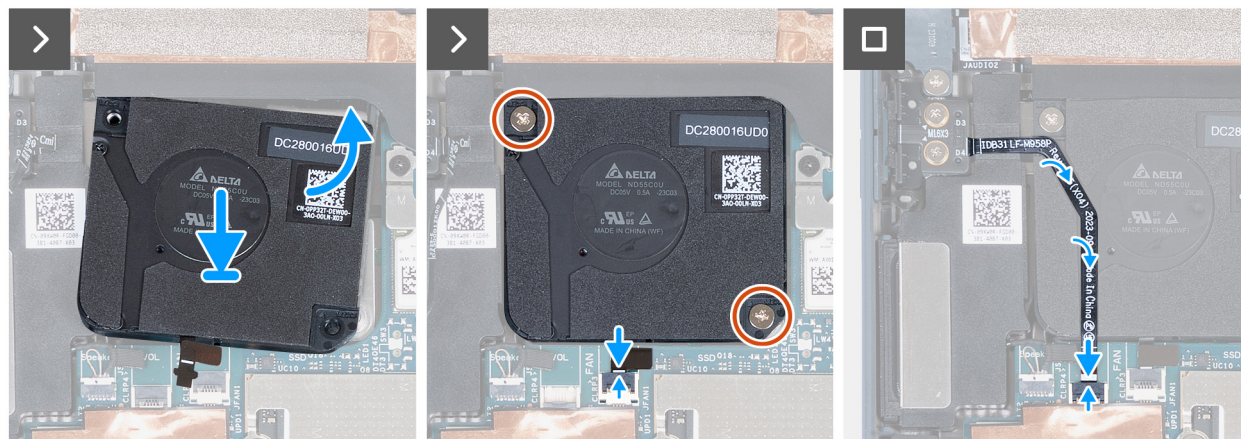
Figure 35. Installing the left fan
