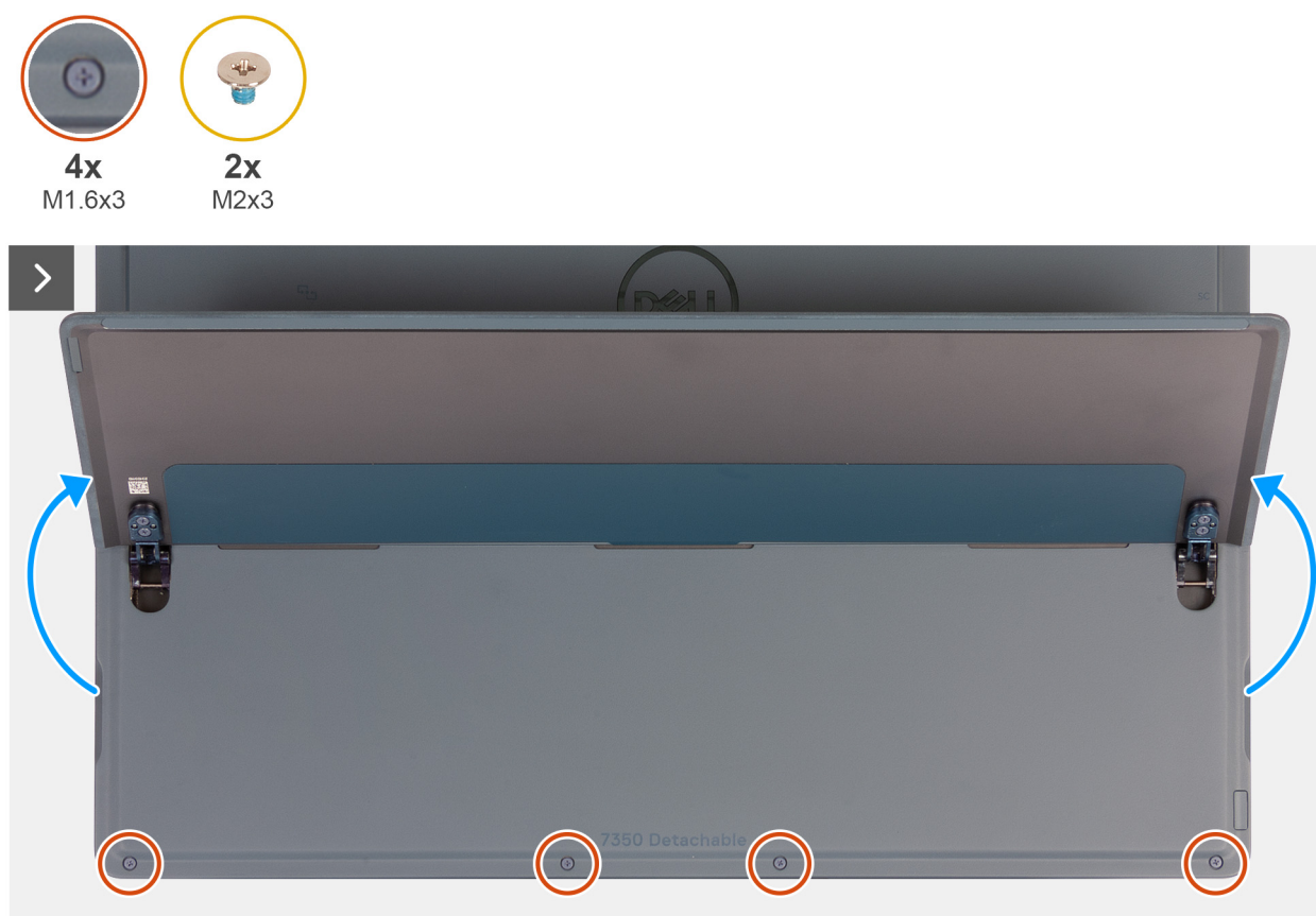
Figure 16. Removing the display assembly
