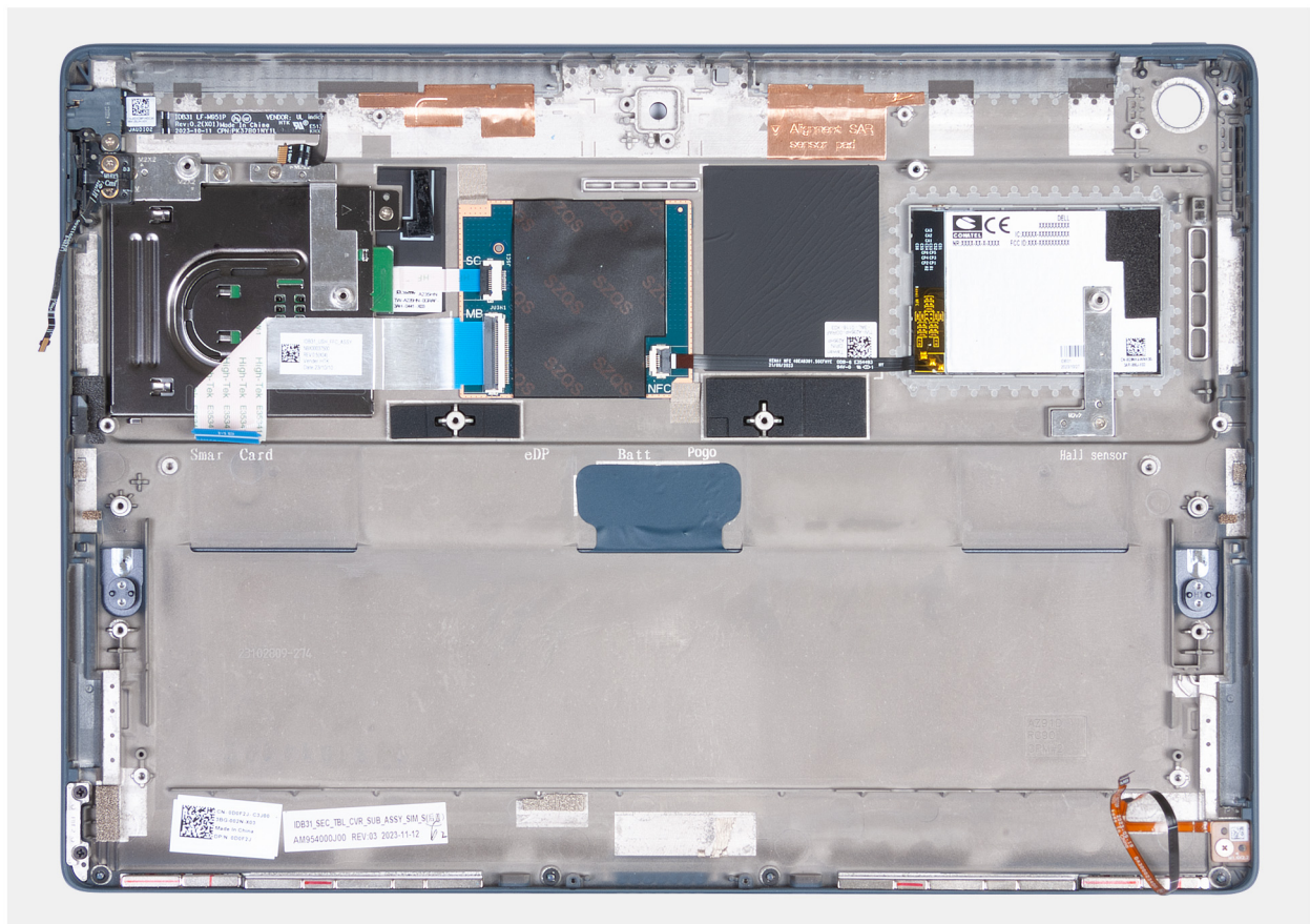
Figure 77. Removing the display-back cover
