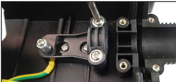
Figure 1-7: Remove the upper clamping
