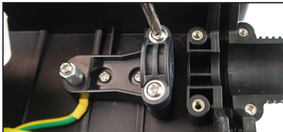
Figure 1-23: Remove the press clamping
