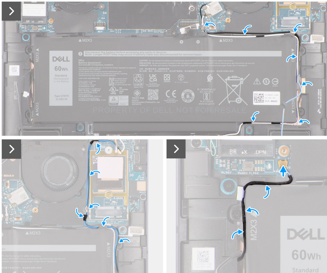
Figure 41. Installing the battery
