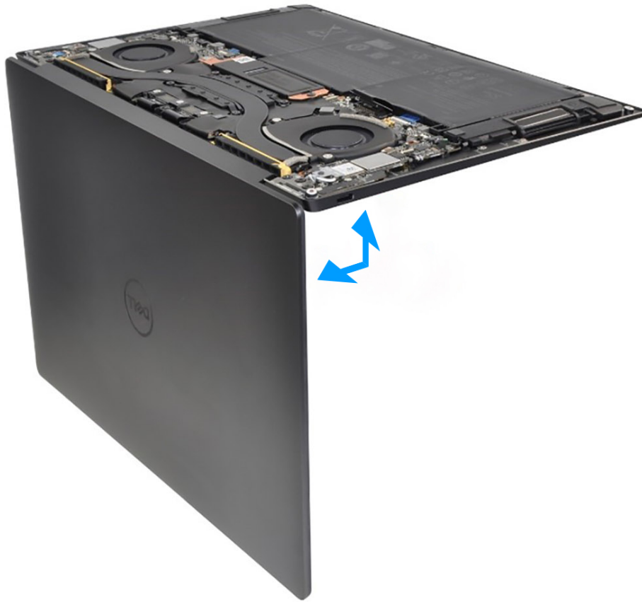
Figure 54. Opening the display assembly to a 90-degree angle
