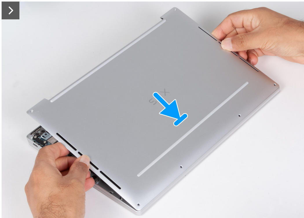
Figure 17. Installing the base cover
