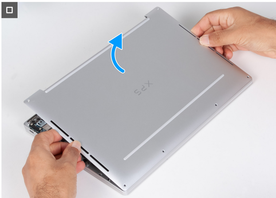
Figure 16. Removing the base cover
