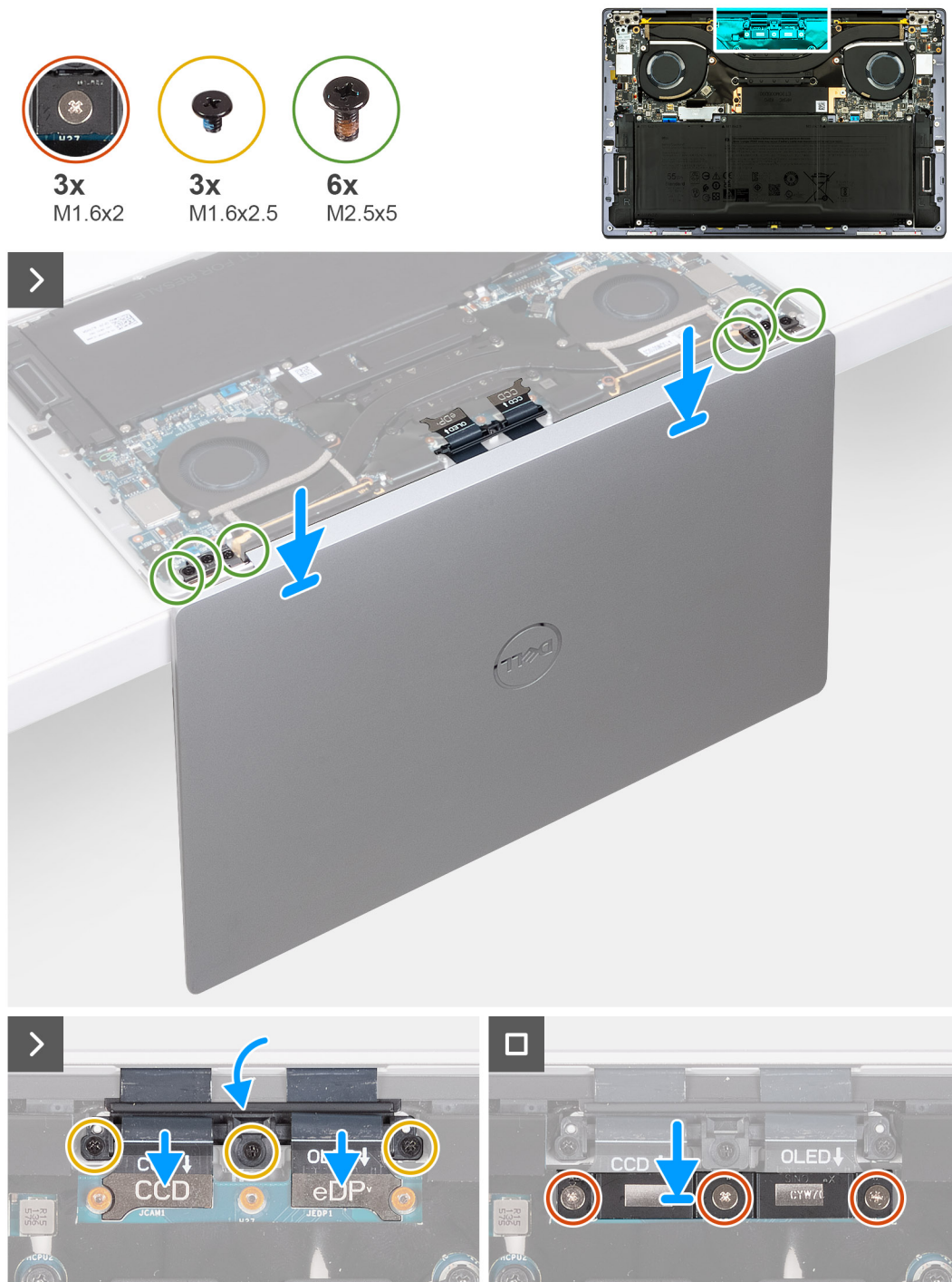
Figure 36. Installing the display assembly
