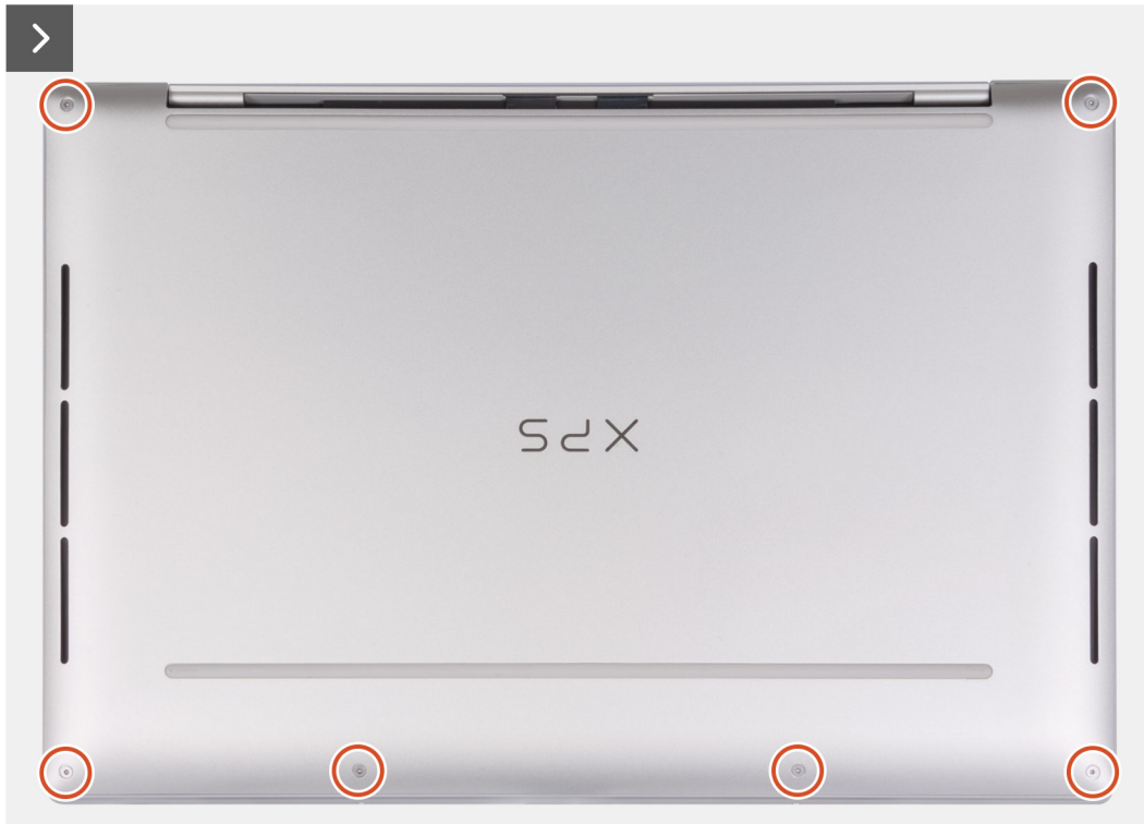
Figure 14. Removing the base cover
