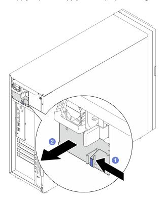
Figure 90. Removing a hot-swap power supply filler
