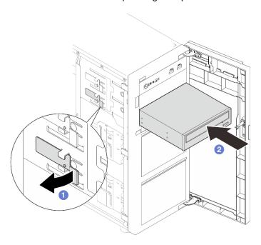
Figure 76. Installing an optical drive
