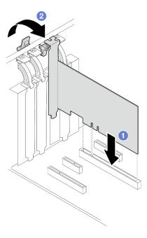
Figure 78. Installing a PCIe adapter
