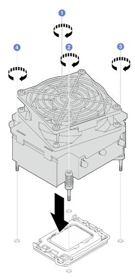
Figure 53. Installing the heat sink and the fan module
