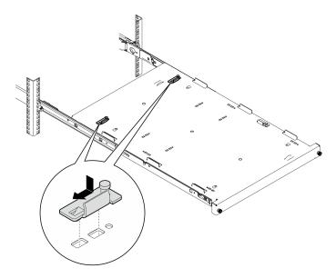
Step 4. Install the four rubber safety pads as illustrated.
