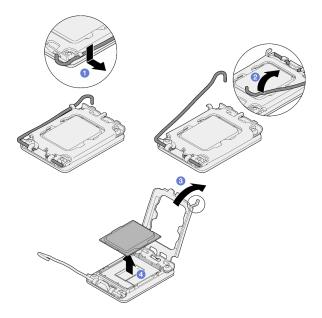
Figure 92. Opening the processor retainer
