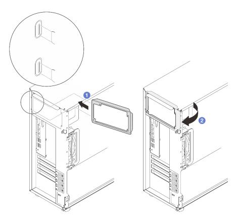
Figure 85. Installing a fixed power supply bracket
