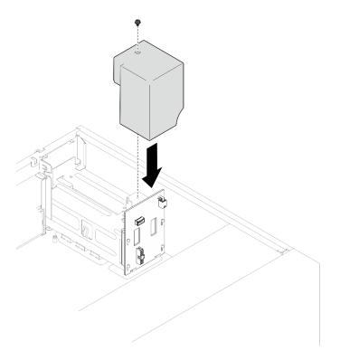
Figure 81. Installing the power distribution board cover
