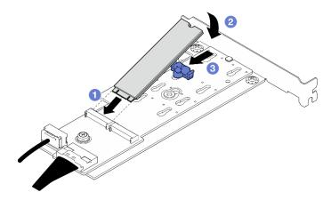
Figure 66. Installing an M.2 drive
