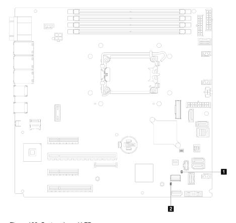
Figure 129. System-board LEDs
