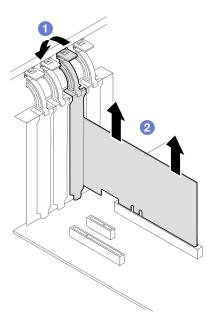
Figure 77. Removing a PCIe adapter
