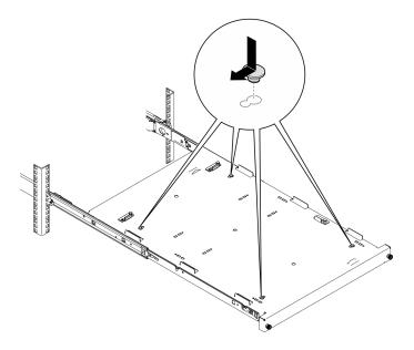
Step 5. Remove the four screws and feet from the server.
