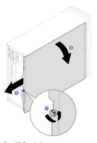
Figure 100. Removing the server cover
