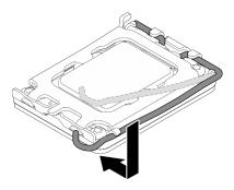
Figure 94. Closing the processor retainer
