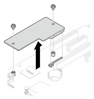
Figure 103. Firmware and RoT security module removal
