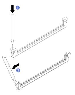
Figure 68. Opening retaining clips
