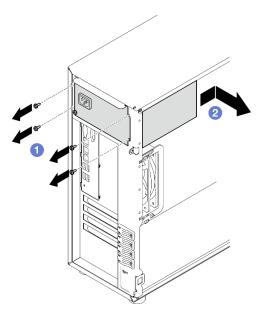
Figure 83. Removing a fixed power supply
