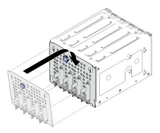
Figure 27. Installing the simple-swap drive backplate
