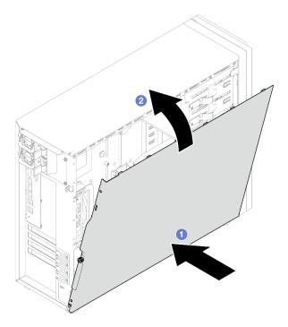
Figure 101. Positioning the server cover onto the chassis
