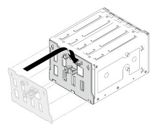
Figure 24. Installing the hot-swap drive backplane
