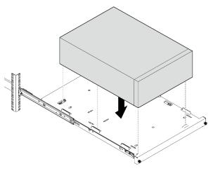
Step 7. Install the server into the rack cabinet.
