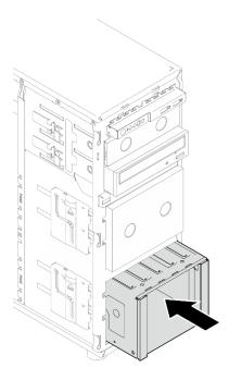
Figure 21. Installing the drive cage
