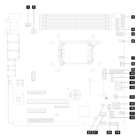
Figure 115. System-board connectors
