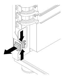
Figure 54. Removing the intrusion switch
