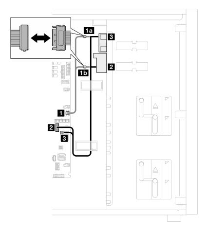
Figure 121. Cable routing for optical/tape drives
