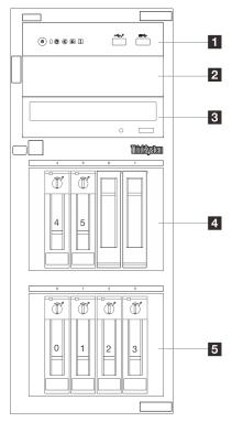
Figure 3. Front view of server models with six 3.5-inch simple-swap drives bays
