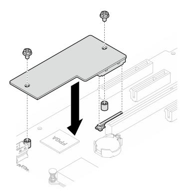
Figure 104. Firmware and RoT security module installation
