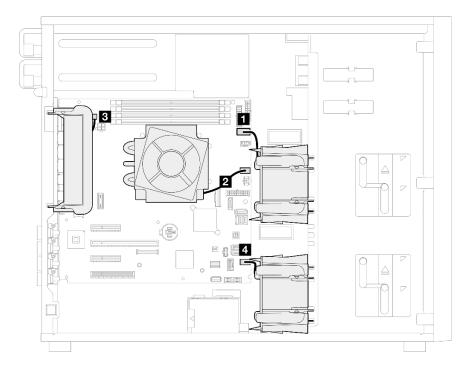
Figure 116. Fan power cable routing
