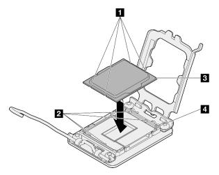
Figure 93. Installing the processor
