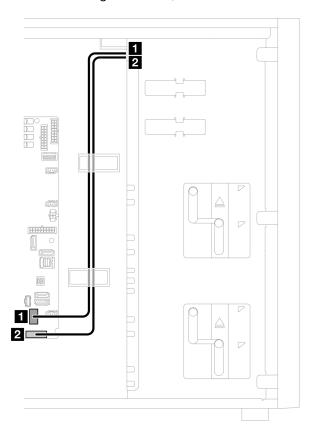
Figure 117. Cable routing for front I/O module
