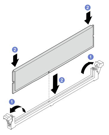
Figure 72. Installing a memory module
