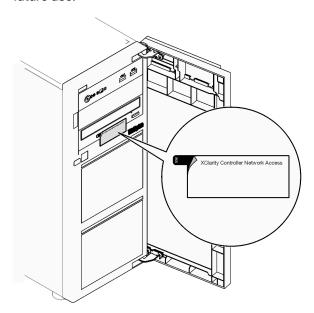
Figure 16. Location of XClarity Controller network access label
