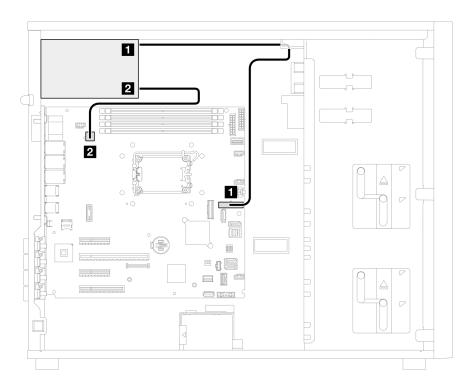
Figure 122. Cable routing for the fixed power supply
