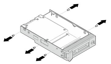
Remove the two screws that secure the 2.5-inch drive; then, lift the drive to remove it from the drive Step 4. adapter.
