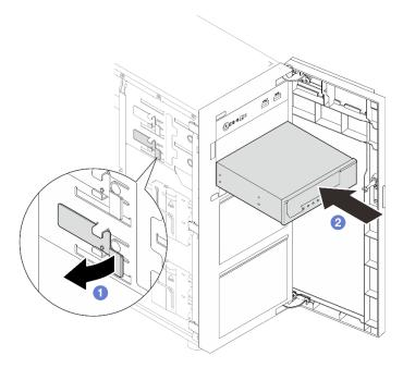
Figure 109. Installing a tape drive
