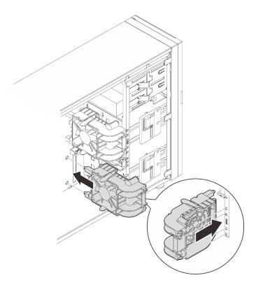
Figure 42. Installing the front system fan
