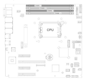
Figure 18. Memory modules and processors layout
