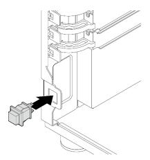
Figure 55. Installing the intrusion switch
