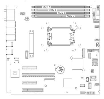
Figure 70. Memory module slots on the system board
