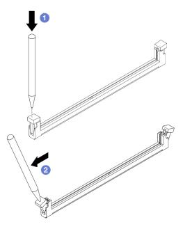
Figure 71. Opening retaining clips
