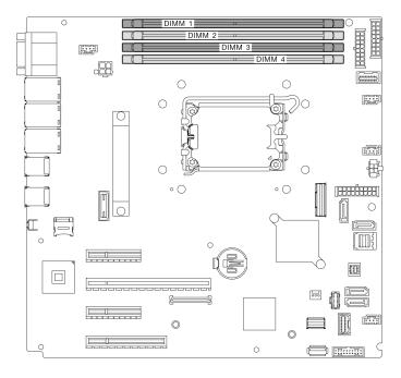
Figure 67. Memory module slots on the system board
