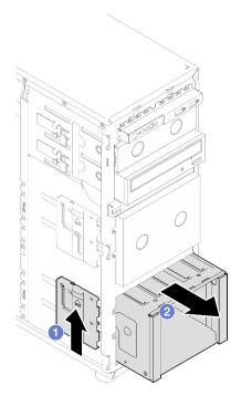
Remove the backplane or backplate. See "Remove the 3.5-inch/2.5-inch hot-swap drive backplane" on page 52 or "Remove the 3.5-inch simple-swap drive backplate" on page 56.
