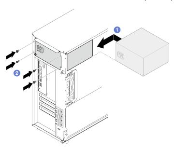
Figure 86. Installing a fixed power supply
