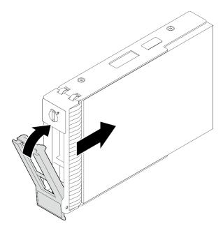
Figure 35. Installing the simple-swap drive
