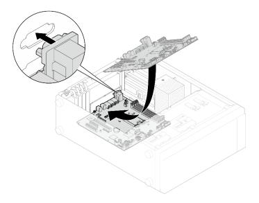
Figure 106. Installing the system board
