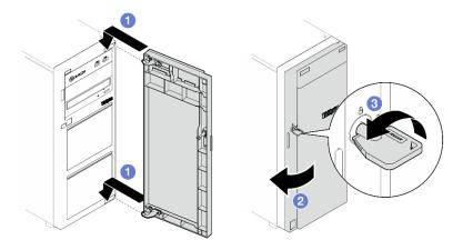
Figure 49. Installing the front door
