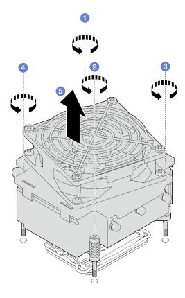
Figure 52. Removing the heat sink and fan module
