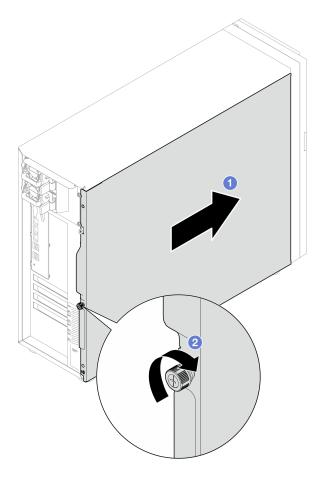
Figure 102. Securing the server cover to the chassis
