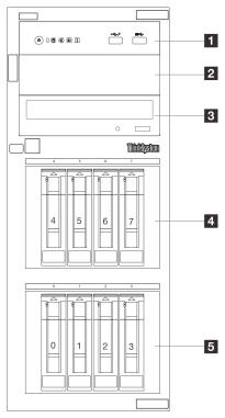
Figure 4. Front view of server models with eight 3.5-inch hot-swap drives bays
