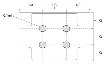
Figure 95. Proper shape of the thermal grease
