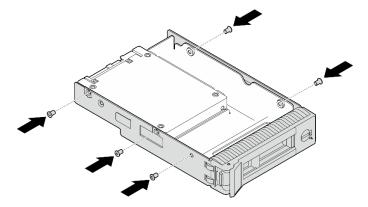
Figure 40. Installing the screws to secure the drive adapter and the drive to the drive tray
