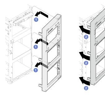
Figure 47. Installing the front bezel
