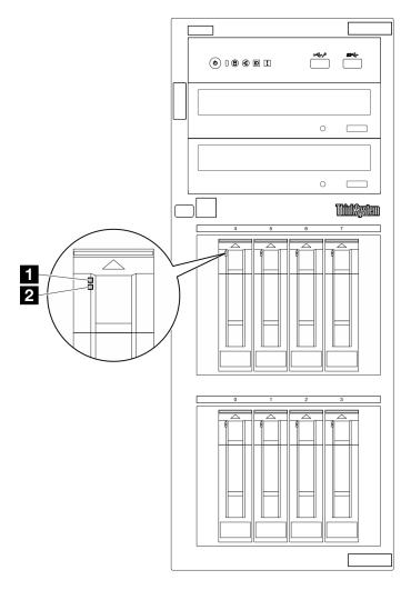
Figure 126. Drive LEDs
