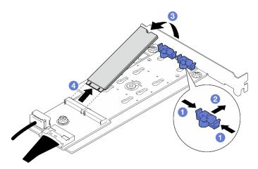
Figure 63. Removing an M.2 drive
