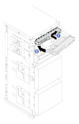
Figure 51. Installing the front I/O module
