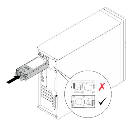
Figure 91. Installing a hot-swap power supply
