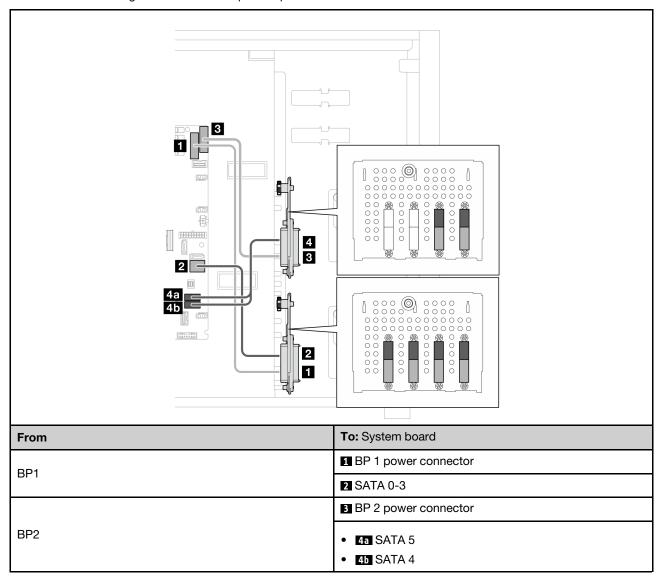
Table 27. Cable routing for optical/tape drives
