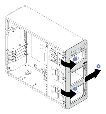
Figure 46. Removing the front bezel
