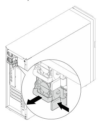
Figure 88. Removing a hot swap power supply
