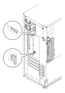
Figure 45. Installing the rear system fan
