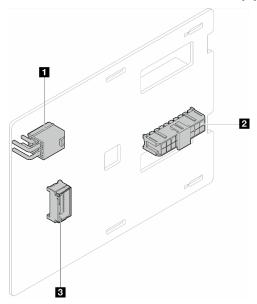
Figure 110. Power distribution board for hot-swap power supplies
