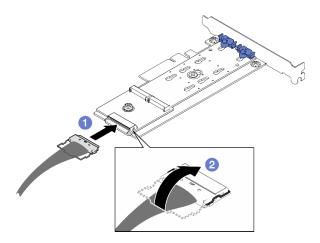
Figure 62. Connecting cable to ThinkSystem M.2 RAID B540i-2i SATA/NVMe Adapter
