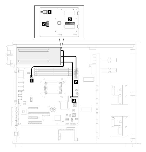
Figure 123. Cable routing for the redundant power supplies
