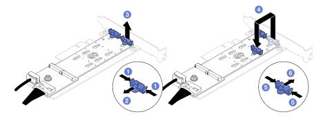
Figure 64. Adjusting the M.2 retainer
