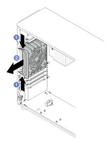
Figure 43. Removing the rear system fan
