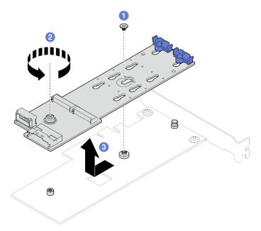
Figure 58. Removing the M.2 boot adapter
