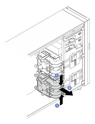
Figure 41. Removing the front system fan
