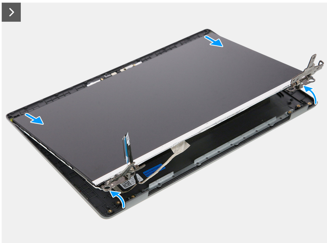
Figure 56. Removing the display panel
