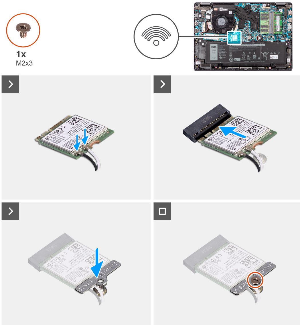
Figure 16. Installing the wireless card
