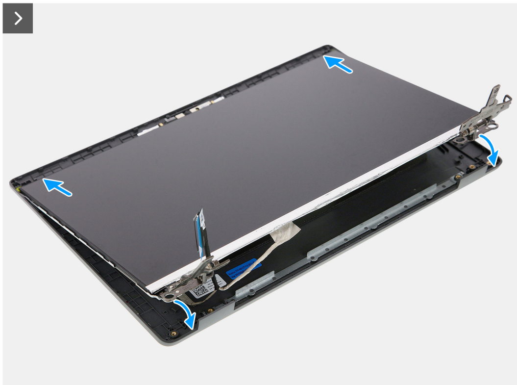
Figure 61. Installing the display panel
