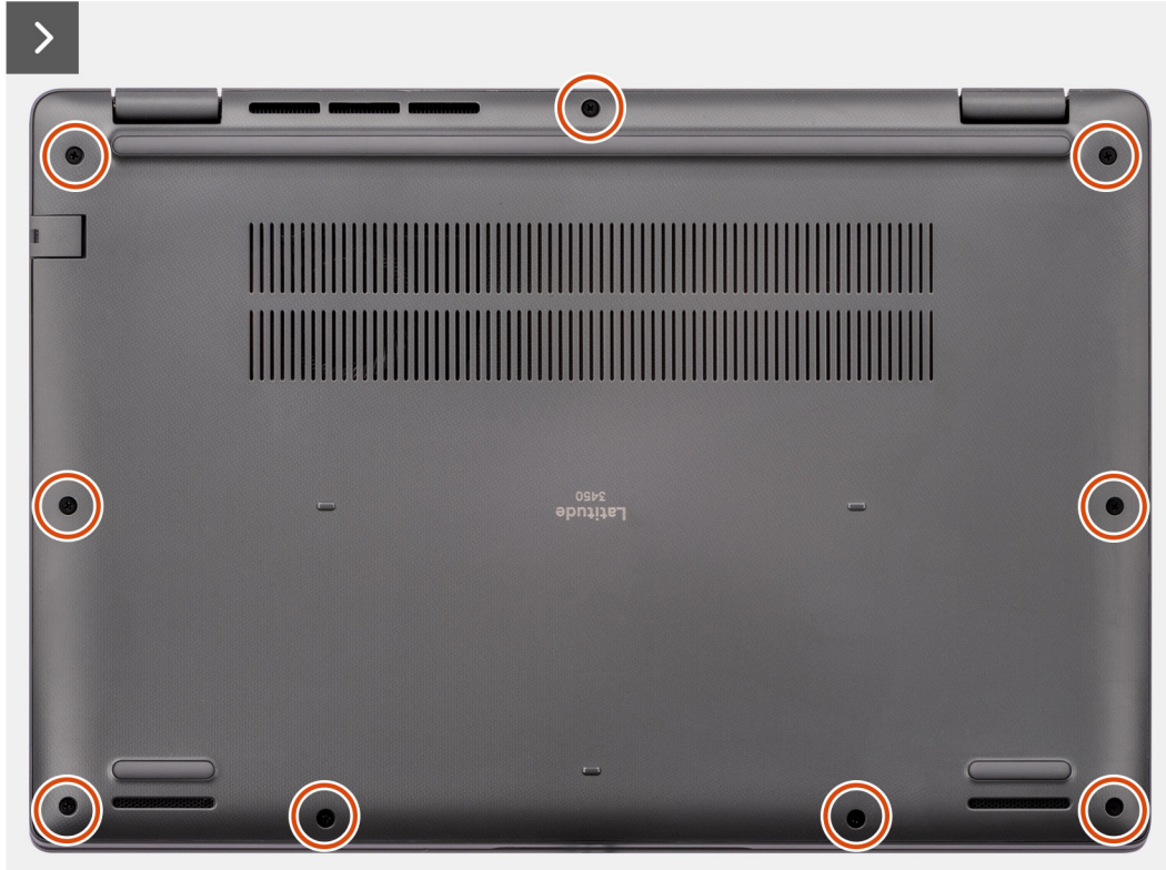
Figure 9. Removing the base cover
