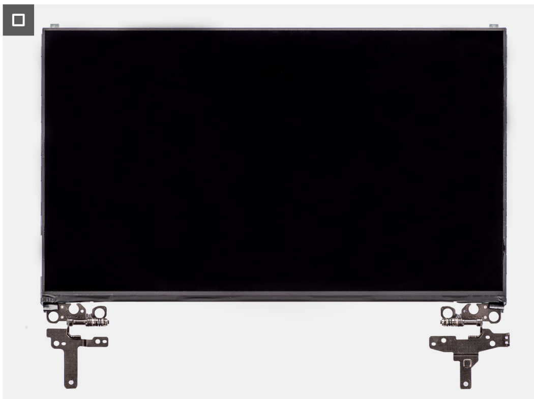
Figure 58. Removing the display panel
