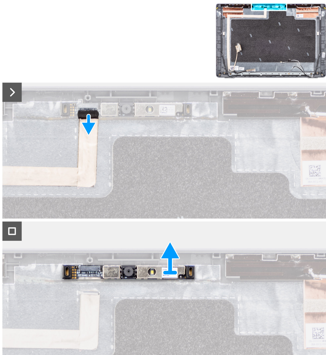
Figure 64. Removing the camera
