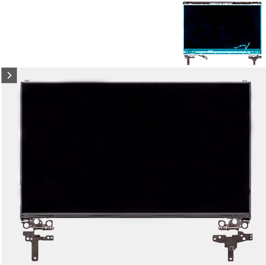
Figure 59. Installing the display panel
