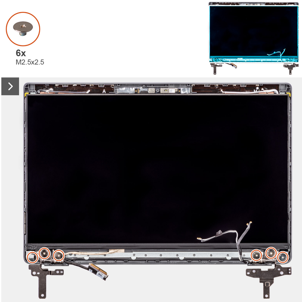
Figure 54. Removing the display panel
